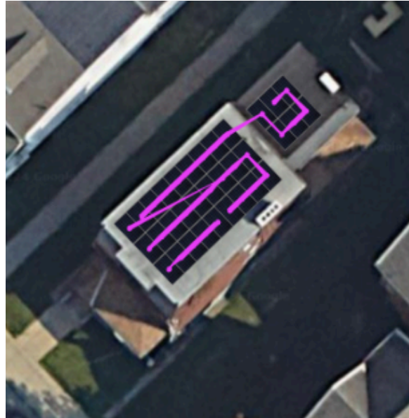
Figure S.3 - Model of solar alternative 3, given by OpenSolar. The pink lines represent the panel connections to one another, also called strings.
