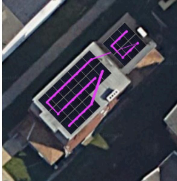
Figure S.2 - Model of solar alternative 2, given by OpenSolar. The pink lines represent the panel connections to one another, also called strings.
